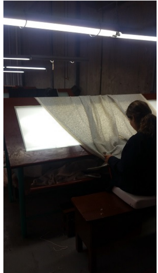
Checking on the light table for flaws
